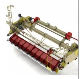
This equipment is equipped with a set of mechanisms and automatisms, the purpose of which is to laterally deposit a pile of sawdust. This unloading robot is mounted in a mobile position on guide rails, inside a building dedicated to its use.
