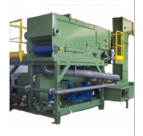
The FLDI filter for cleaning fluids has several advantages such as operational reliability. The filtration capacity is estimated from 5 to 25 m3 / h.
