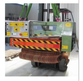
This special machine was made to turn beams of 30 tiles ref: DC12 1 UG strapped and well stacked. The tile turner has excellent clamping and lifting capacity. There is possibility of rotation of the beam on 180 °
